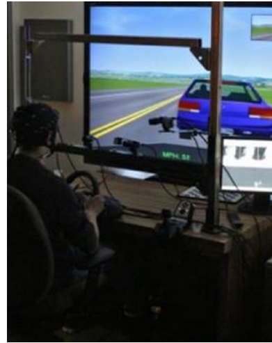
Figure 1. Experimental setup of the DriveSafety simulator and SmartEye tracker.
