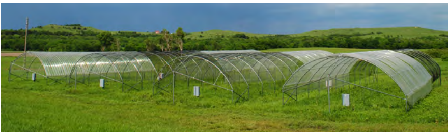
FIGURE 4.3 The climate extremes experiment at the Konza Prairie Biological Station. Experimental manipulations of precipitation using large rain-out shelters allow ecologists to test the predictions of climate change on intact grassland communities. Image credit: Melinda D. Smith.
