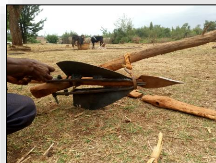
The wooden wings of the traditional animal drawn implement is replaced by metal, which is aimed at reducing the number of repeated plough during seed bed preparation and the reducing the amount of weed. Photo credit: Yonas Degu.
