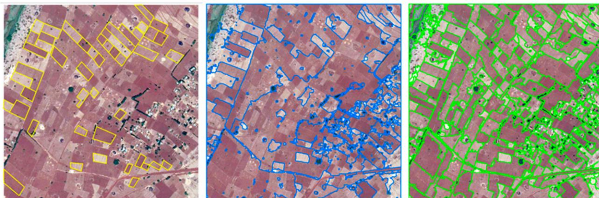
Reference boundaries (a) and outputs from the two boundary detection methods, gPB (b) and eCog (c), for one 1 km × 1 km tile in the Amhara Region
