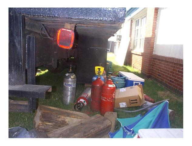
Violation: Improper storage of compressed gas cylinders.
