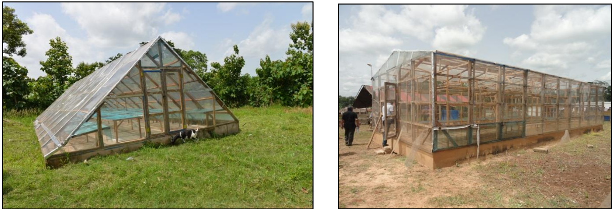
Figure 6. Multi-crop solar dryers with mesh covered racks seen in the Middle Belt of Ghana (near Nkoranza on left and Sekyedomasi on right) during our assessment trip.
