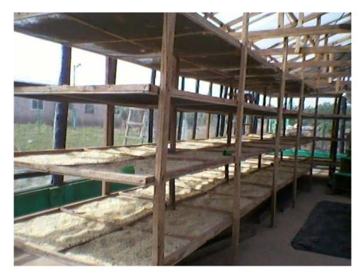
Figure 2: Shelves stacked with maize harvest in the biomass hybrid solar dryer in Ejura, Ghana.
