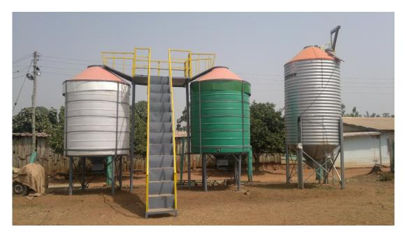
Figure 3: Plastic water tanks modified into silo for long term storage of maize in Ejura, Ghana (metal silos on the right was donated from a Brazilian company and additionally tested).
