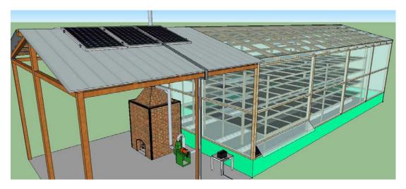
Figure 1: Schematic diagram of the biomass hybrid solar dryer set up in Ejura, Ghana.
