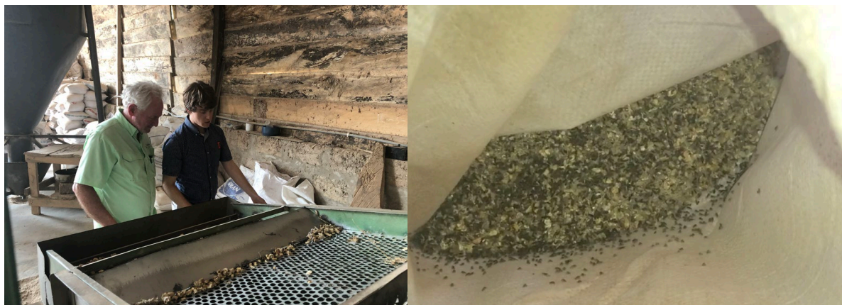
Photo: Drs. Paul Armstong (USDA-ARS) and Matt Stasiewicz (University of Illinois) discuss a locally innovated maize kernel sorter at EwanJoes farm (R), and the waste stream that has been sorted out, ridden with weevils since the sorted maize had not been stored in a hermetic bag.
