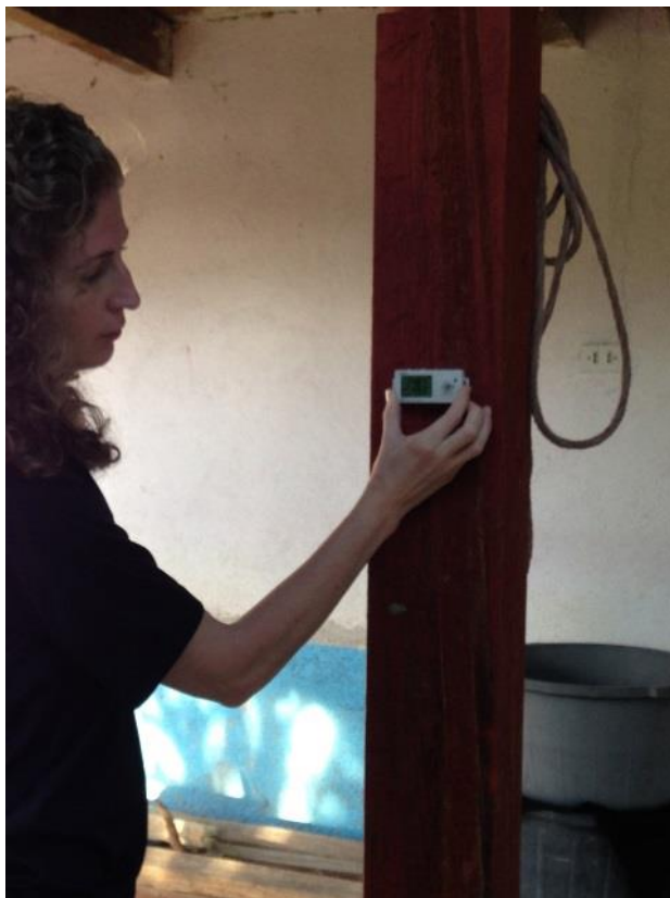
Measuring ambient temperature & relative humidity conditions during storage
