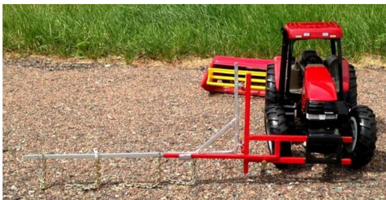
Figure 12. A photograph of flushing bar on a mower used in pollinator habitat (taken from Biodiversity Management Guide).
