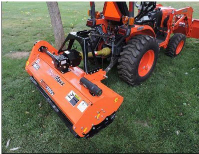
Figure 13. A photograph of a flail mower used for managing pollinator habitat (taken from WoodMax Power Equipment)
