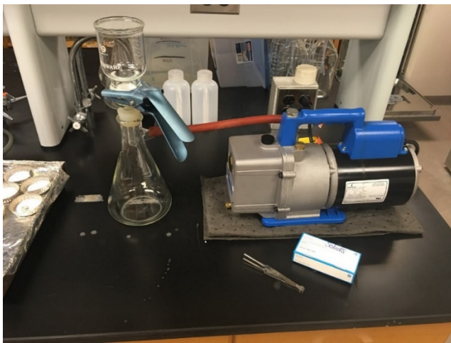
Figure 22: Suction Pump Used for Solids Filtration
