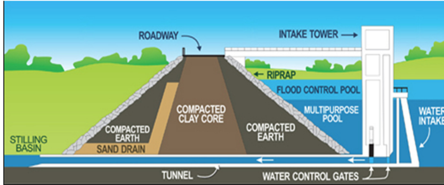
Figure 8: Bottom Controlled Reservoir Outlet Structure (Osage County, 2018)
