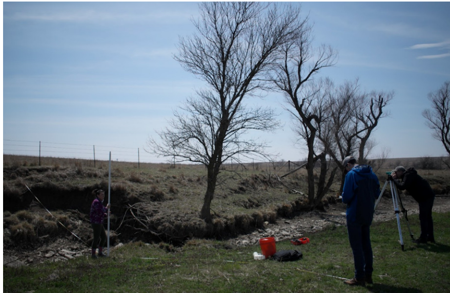
Image 3: Taking stream profile measurements using a level sight and leveling staff.
