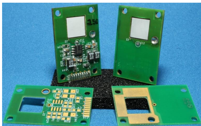
Fig. 3. Shown are dual-integrated packaged devices with preamplifying circuitry. The motherboard, which provides an adjustable detector bias, bias current compensation, pulse shaping and gain, an analog output for pulse-height analysis, and a “digital” output from a discriminator, is show elsewhere [7].
