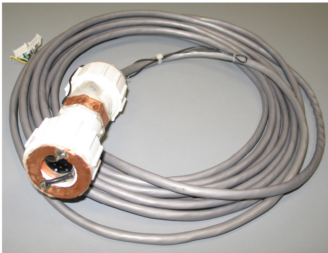
Fig. 2. Encapsulated data acquisition hardware and cable.
